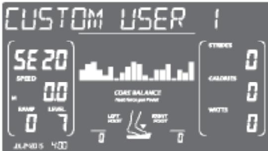
Once the program has been set up, simply scroll to the USER1 or USER2 program and press Start. Both Ramp and Level are shown in the program matrix with the Ramp on the left and the Level on the right.
